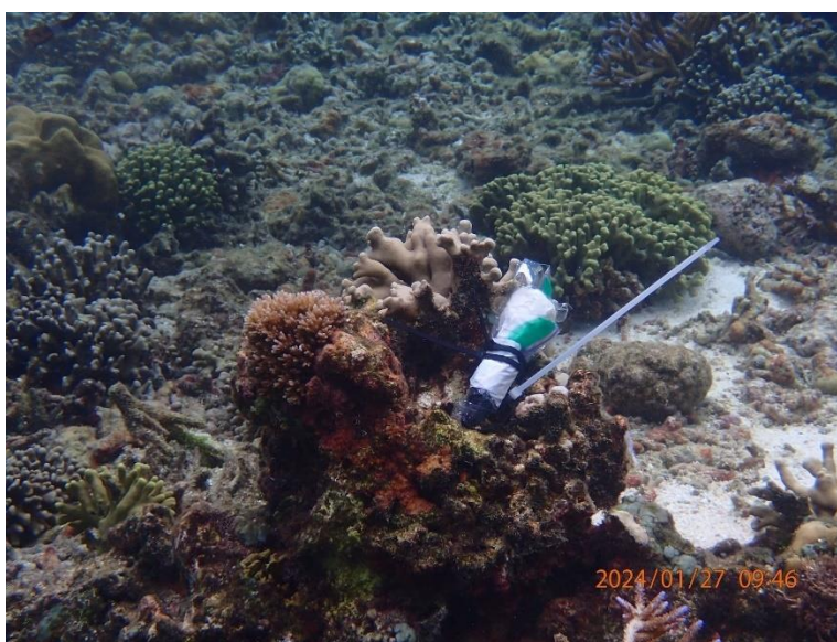
Figure 12. Demonstration of a HOBBO logger attached to a coral with a zip tie.
