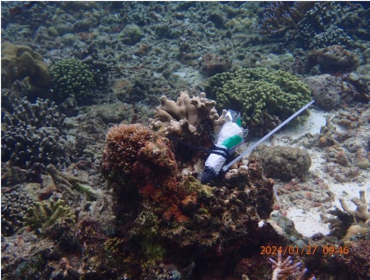
Figure 13. Demonstration of a HOBOT logger attached to a coral with a zip tie.
